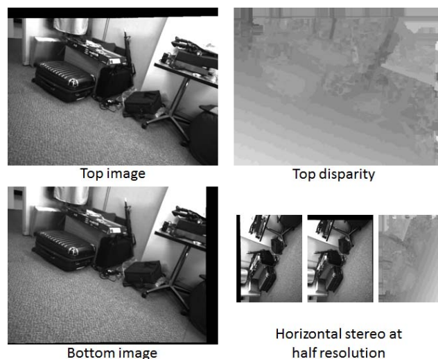
Figure 6: Real time stereo processing example. Vertical stereo feed is transposed as a horizontal stereo pair.
